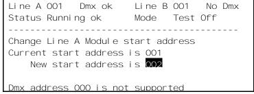
You can set the start address for DMX line B by using the DMX B button in the same way.
