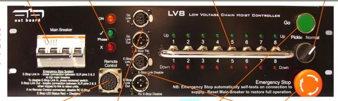
Remote operation of the LV8 is available using the optional RC8 remote control handset, which provides Up/Down switches for motor direction, GO and E-Stop. The RC8 handset is connected to the LV8 via a detachable multicore cable. Two LV8's can be run from one RC16 sixteen-channel handset via an RC Handset Splitter. Programmable control systems such as the IBEX PHC+ can also connect to this Remote Control socket to automate the LV8.
