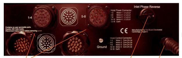
Connections to hoists are arranged in groups of four channels on 19-way Socapex connectors. Female carries four channels of 3-phase power/earth, Male carries four channels of Up/Down control.
