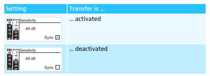
By pressing the symb button 3, you can transfer the parameters to the transmitters via the infra-red interface (see page 22).
