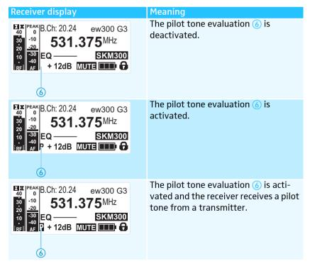
Devices of the ew 300 G1 series (generation 1) do not support the pilot tone function. Therefore, please observe the following when combining a radio microphone or receiver of the ew 300 G3 series (generation 3) with devices from an earlier evolution wireless generation:
