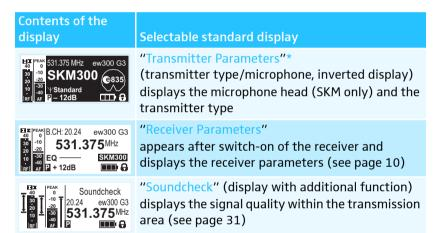
\* The reading of the transmitter parameters can take up to 2 minutes. If you synchronize your transmitter with the receiver (see page 22), the parameters are read out without delay.
